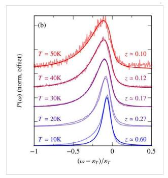
The new technique shows remarkably good agreement with experimental results, essentially perfect at high temperature, with small discrepancies at lower temperatures. Comparison of theoretical (solid dark) and experimental (solid light) photoluminescence spectra at different lattice temperatures. 'perturbatively' exact theory (referring to a quantum system being perturbed from a simple, solvable limit).
