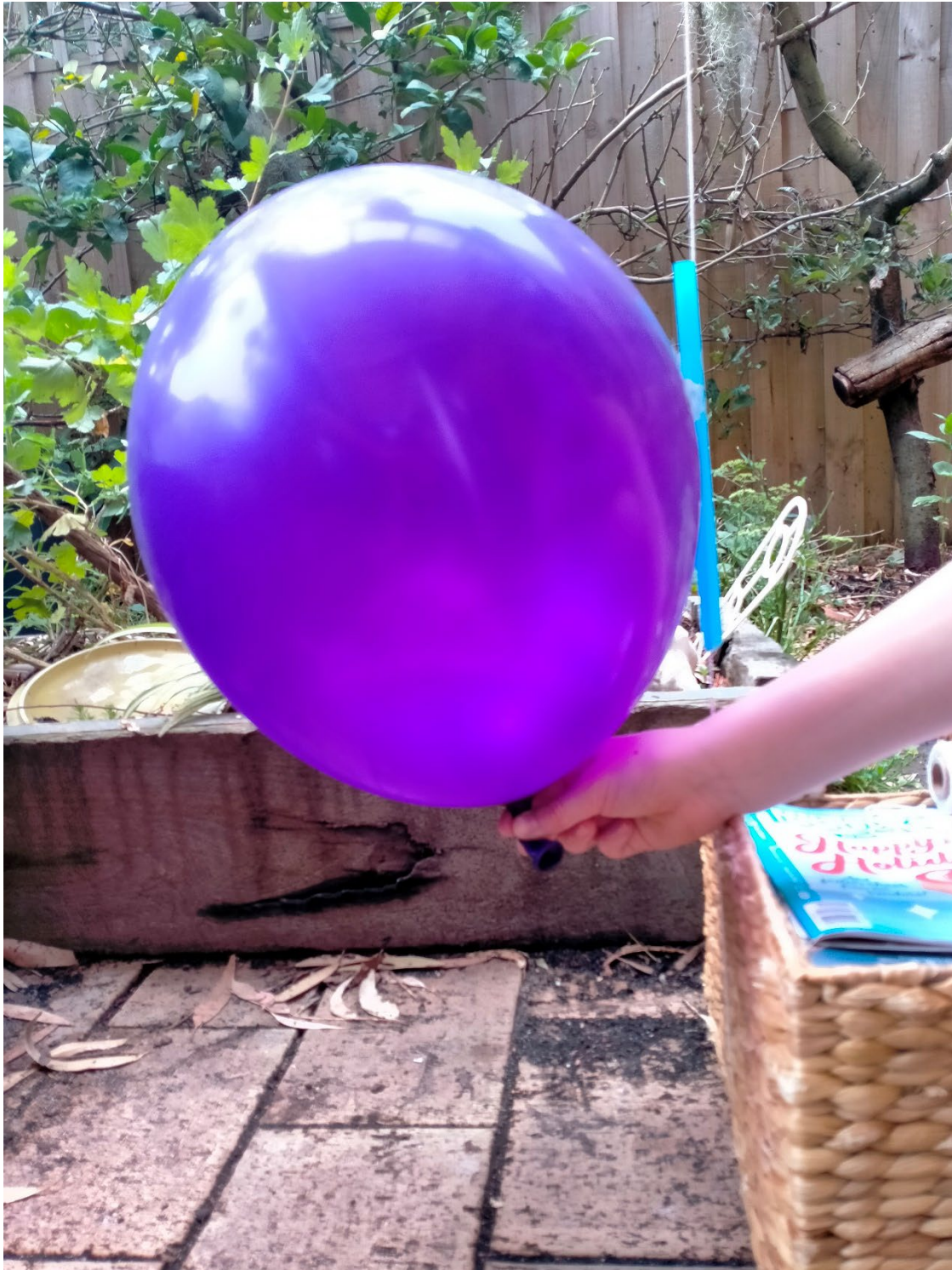
Figure 3. The countdown before launch of the balloon rocket on the vertical string. As in experiment 1, the balloon is taped to the straw that enables the balloon to travel up the string – if there is enough thrust.
