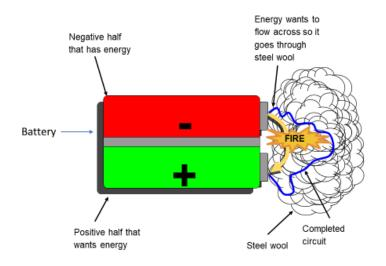
Figure 1. In a fully charged battery, the negative half of a battery is where all the electrons are stored. The other half stores positively charged ions. When you create a circuit between the two halves of the battery, the negative electrons will want to move through the circuit to the positive terminal. The resistance the electrons meet on their journey through the extremely thin steel wool circuit create sufficient heat to cause the thin wool wire to catch fire. Image by Tristian Fuhrer.
