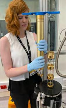
A new low-temperature fridge installed in the FLEET labs at UNSW will allow study of 2D systems in advanced semiconductor devices.
