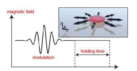
An oscillating magnetic field is applied to an atomic gas (shown upper right), causing it's size to oscillate in two dimensions.
