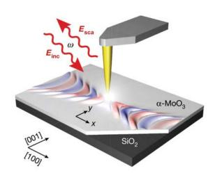
Near-field optical microscopy is a new method allowing improved imagery of polaritons.
