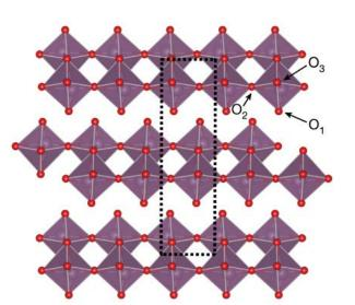
The structure of molybdenum trioxide is distorted by vdW interactions.
