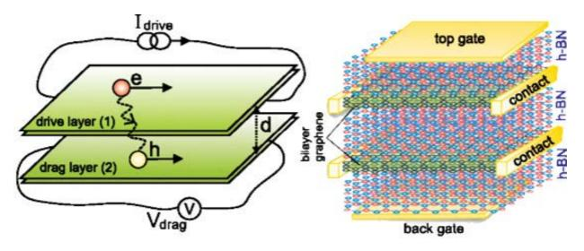
Left: An electron (e) accelerated in the top sheet causes a hole (h) in the lower sheet to be accelerated.
