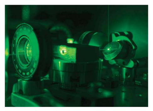
Laser equipment (532nm) at Swinburne University of Technology, used to confine the atomic gas.
