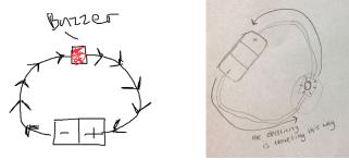
*Correct circuit, incorrect electron flow:* Student drew a circuit correctly but labelled the electrons flowing from the positive to the negative battery terminals
