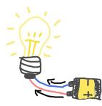
*Correct and with series/parallel circuits:* Some students had set up functional circuits in series and parallel. Students noticed that lights, buzzers or motors were dimmer, or weaker when set up in a series.
