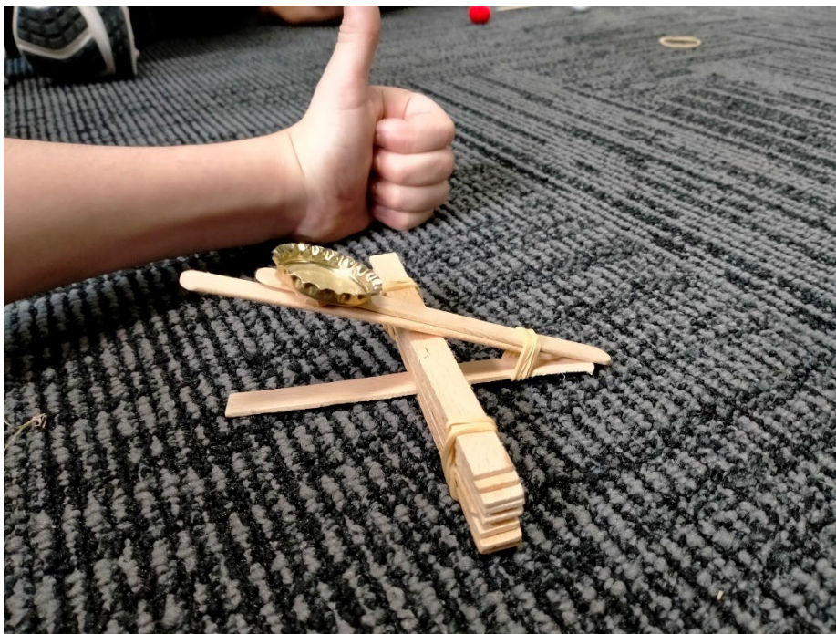
Figure 2. Students' later modifications were more successful. Two layer of icy pole sticks increased the strength and potential elastic energy of the lever.
