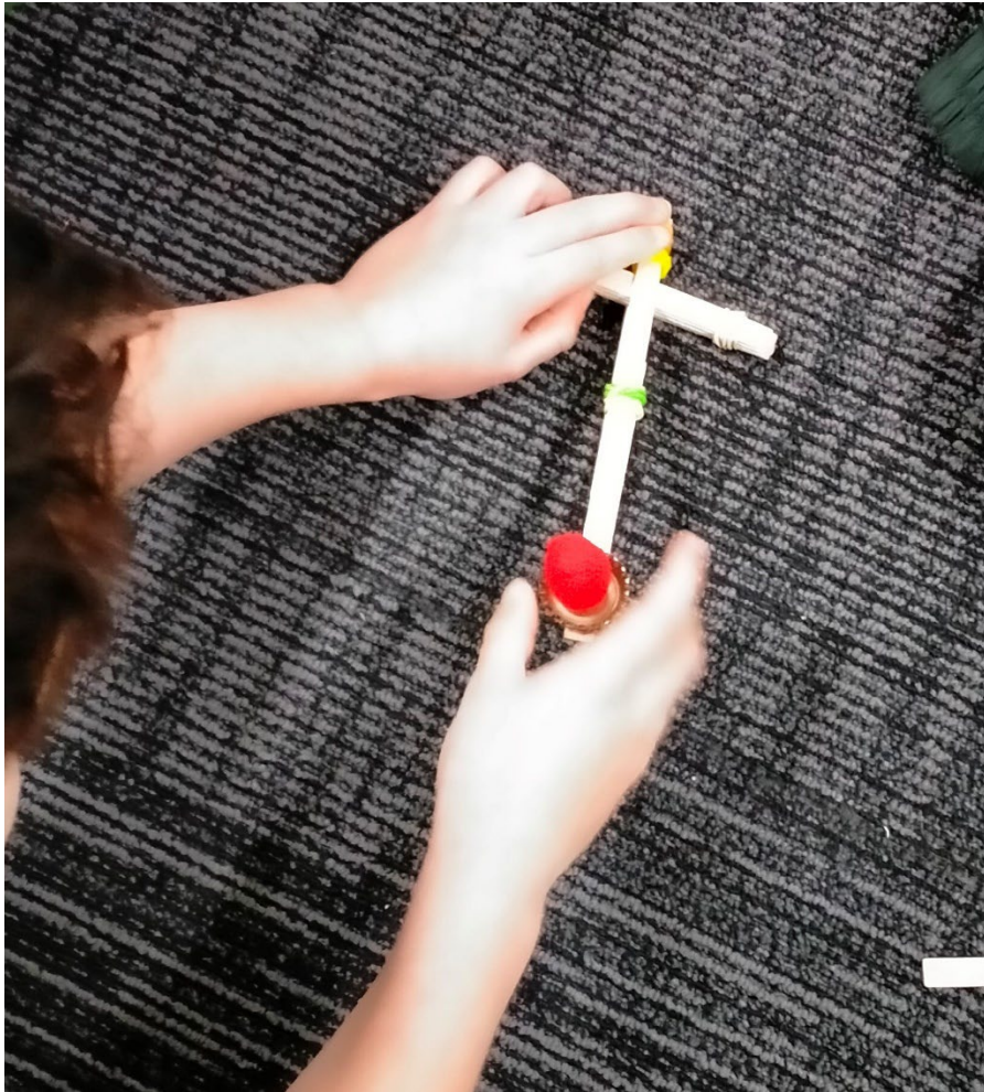
Figure 1 (b) An early modification to increase potential elastic energy to the lever – extended lever modification
